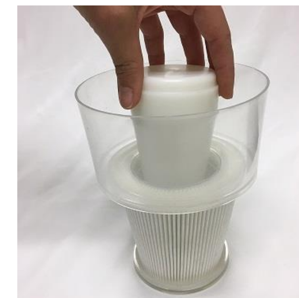
Figure2 Pleated 1.2 µm Glass microfiber with void displacer unit to minimize hold up and improve recovery
