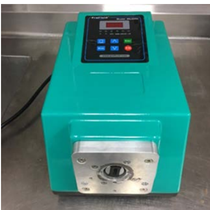
7. front of pump drive unit
