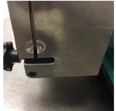
30. This is an insufficiently tightened HemiTor door. Note the gap.
