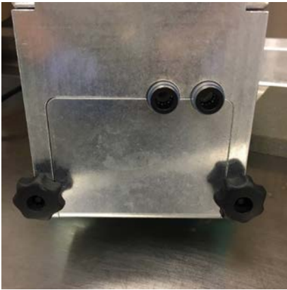
28. the front of the doors should be flush to each other when properly tightened down
