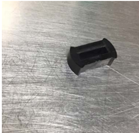
11. motor drive spud adapter (your pump may not have one)
