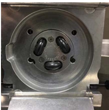
16. Align the notches on the inner hub to align with the mounting screw holes.
