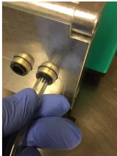
32. Insert the tubing firmly and completely into the fittings. Push to make sure they are securely and completely seated
