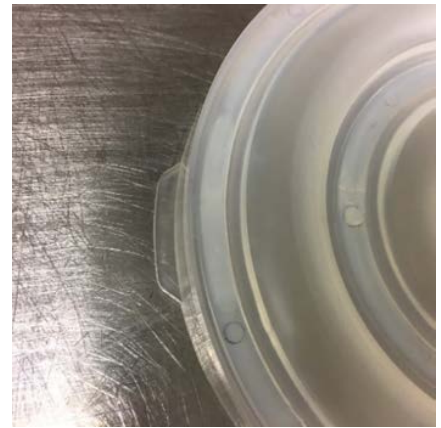
21. mounting orientation tab on the HemiTor cassette insert
