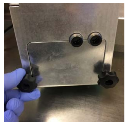
27. Be sure that the knobs are firmly tightened down, failure to do so will cause the pump to lose pressure
