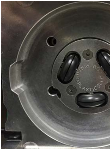
22. Note the location of the notch where the mounting orientation tab fits
