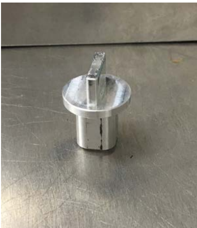
10. close up of the drive spud
