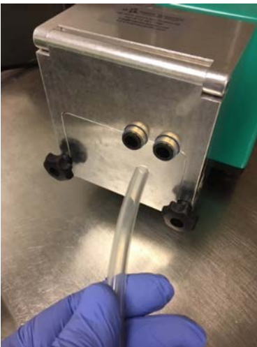
31. Insert the tubing into the quick Disconnect fittings on the pump insert. The inlet port is on the left, closer to the center. The outlet is on the right
