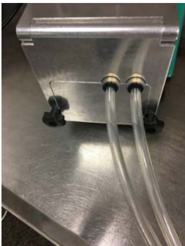
34. Correctly installed tubing in the HemiTor
