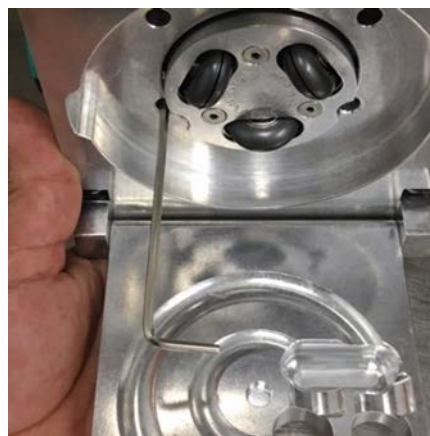
17. Support the HemiTor drive adapter with your hand, insert mounting screws into mounting holes and tighten with the provided hex wrench. Wiggle the screw to make sure it inserts and seats into the screw hole.
