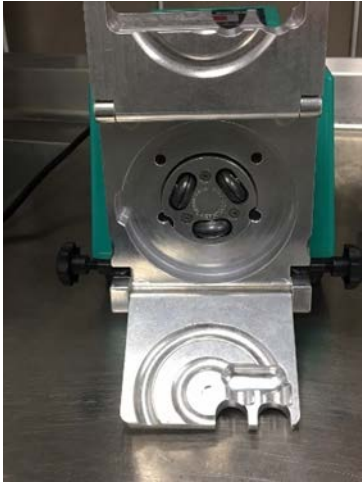
19. properly installed HemiTor drive adapter, with doors open
