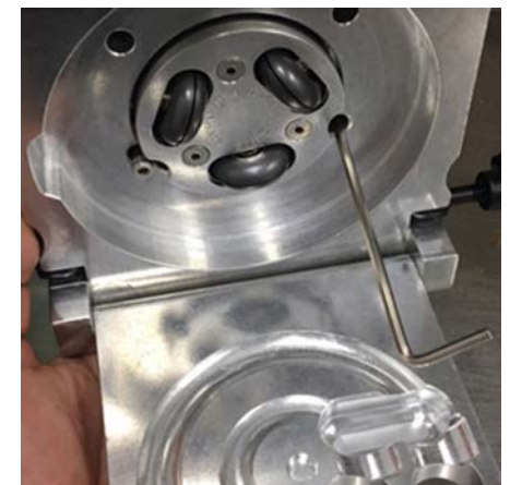
18. Repeat for the other mounting screw. Tighten the screws just tight enough, until they stop
