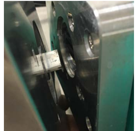
15. When attaching the HemiTor drive adapter to the pump drive, note the orientation of the blade on the spud and make sure it is lined up with the drive.
